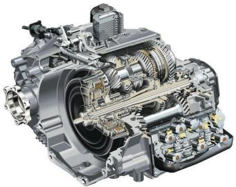
Figure 3: Semi-Automatic Transmission system [3]
