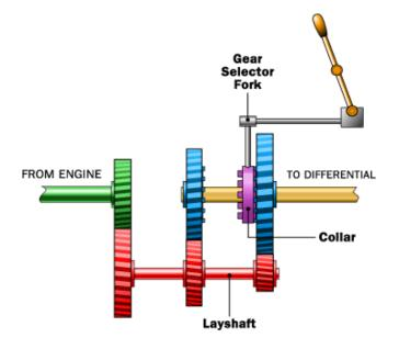
Figure 1: Manual Gear transmission system [4]
