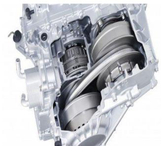
Figure 5: Continuously Variable Transmission system [2]
