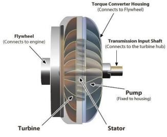
Figure 2: Fully Automatic Transmission system [4]
